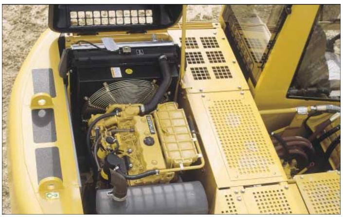
The 3054 TA Engine. Fuel economy at its best. It features a high thermal efficiency and reduced friction resistance between piston and liners.
