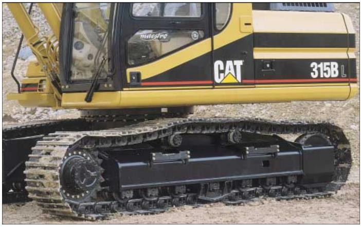
Precision robotic welding helps ensure quality welds. These welds increase rigidity, reduce internal stresses and enhance durability for the chassis and track roller frames.
