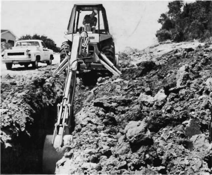
14'-18' (4267 mm - 5486 mm) telescoping Extendahoe provides up to 4' (1219 mm) of extra reach and dig depth.
