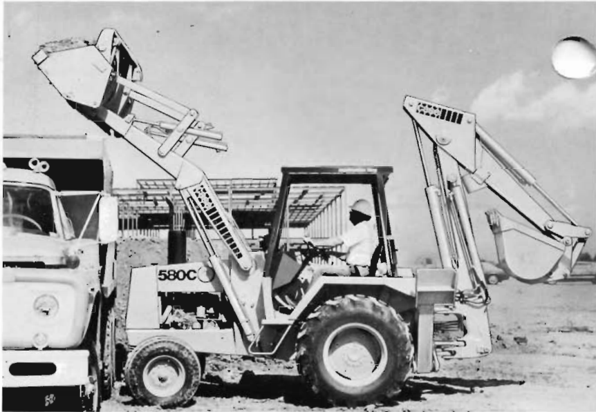
Self-leveling loader keeps payloads moving.
