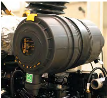
Improved Air Filtration Donaldson Filter
